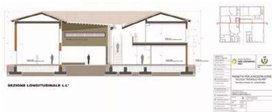
Fig. 8. Project of the new school “Romolo Murri” of Gualdo. Cross section of the open space-cloister in the middle and of the covered space-Agorà. The maximum height are 7.43 m at the eaves extraction and 9.16 m at the top higher (source: L. Notarantonio 22/09/2017).
